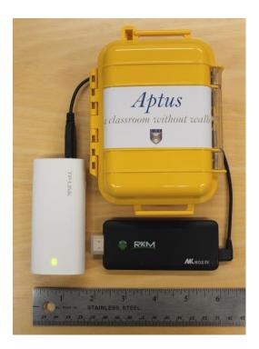
We can re-purpose the Android Mini PC to act as a server capable of hosting content that can be shared via the wireless network with learners. The Android Mini-PC can run effectively on battery power from a power bank (there is one contained in the wireless router) that can be recharged a solar charger. Together these two devices cost just under \$100 and form the core of the Aptus Classroom Without Walls.
